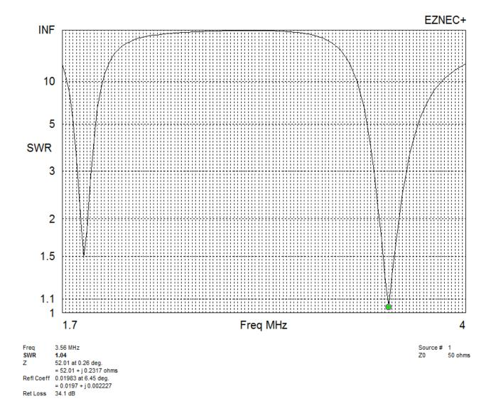
Foolishly thinking it was cautious, the 80m wires were cut to 64' to start, the 160m ends were left quite long and the antenna elevated to the top of the lower 45' of my spiderbeam 18m fiberglass telescoping tubes. Two fiberglass Jackite supports of 25' were (from the old antenna configuration) about 80' from the center support. The first thing noticeable was the substantial droop of the relatively heavy traps.
