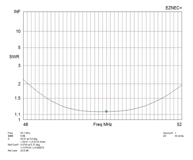
With EZNEC a design was settled on using 3/16 aluminum rods as elements. Later the design went to the use of 1/8 rods for the outer portion of the elements but this has little impact. This plan, for 25' height, has half elements of 59, 57 and 52 inches with a 5" offset of the DE toward the DIR. The individual element resonant frequencies are then, 47.8, 49.5 and 54.4 MHz, but a bit higher at my 10' test height (says EZNEC).
