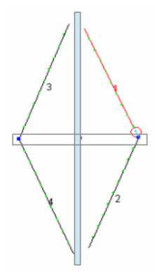
EZNEC is a powerful, though less than perfect, tool for antenna design. However so long as you avoid taking the dimensions as exact, much can be done. In this case numerical experiments with a range of wire lengths and spacing were tested. One major goal is make the raw (unmatched) impedance near 50 + j0 ohms to allow direct coax feed with a tolerable SWR. The principal dimension to control the real part of the impedance is the spacing, or boom length.
