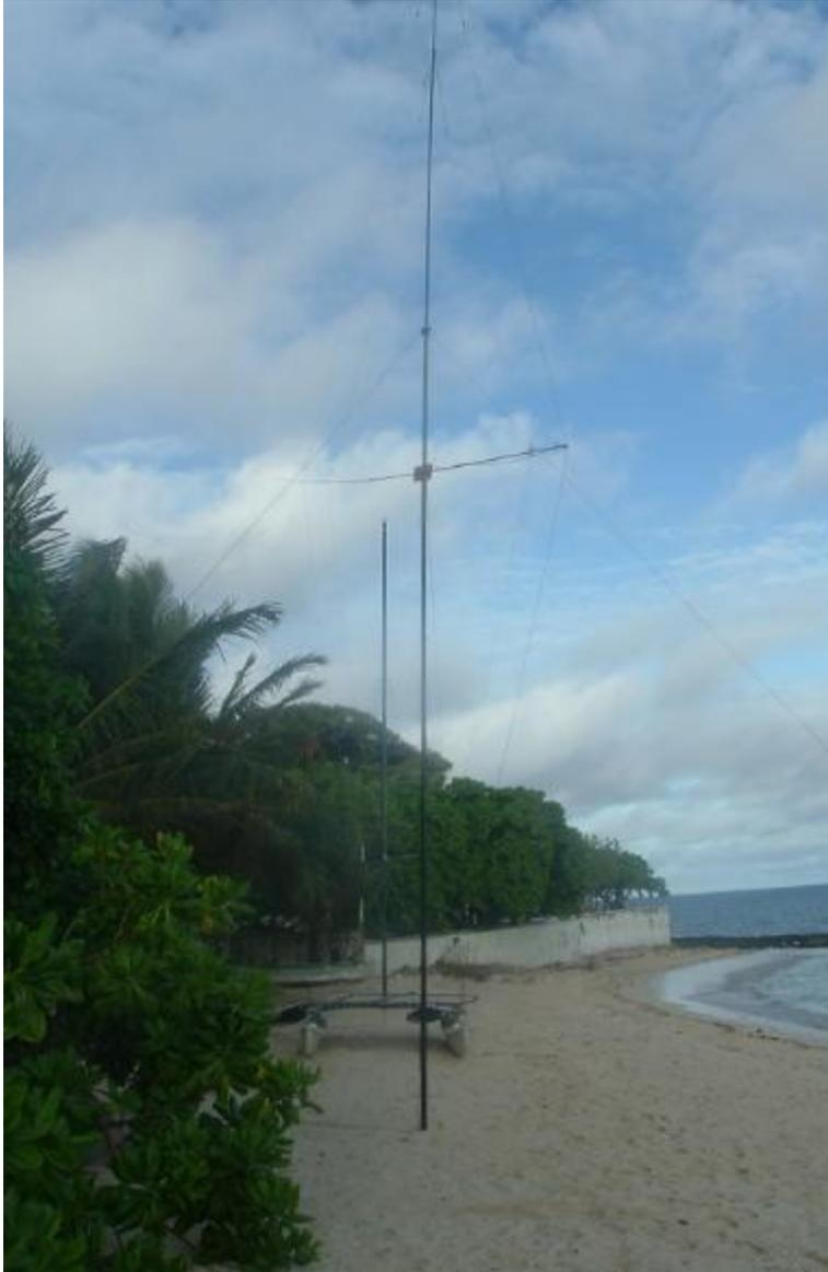
Up with less sleep than desired but it is the day to put up the big vertical for 160/80. First a better evaluation of the location needed for the radials and so the 20/17 VDA will need to be moved west, not a huge deal. Slowly everything is laid out with four guys plus the radial elevation using the jackite poles. The 18m pole goes up with 2 helpers from the hotel and the guys are set, two with sandbags and two at trees.
