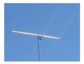
Recently a set of several test antennas were constructed here from a tinker toy set of 8 pieces of 6' telescoping Al tubing (2 each of 3/4, 5/8, 1/2 and 3/8"). These were, in order: a 30 m two el parasitic vertical; a 17 m two el parasitic vertical; a 17m two el yagi; and a gamma match testing 22.1 MHz dipole. Some of these are described in other notes.
