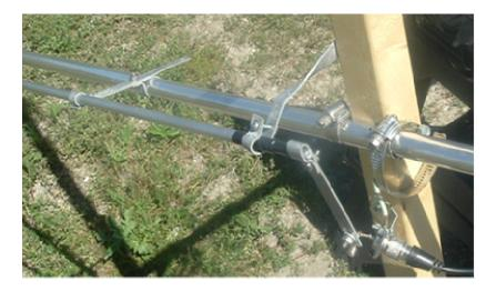
The capacitor is a "gimmick" coaxial type consisting of a short length of 1/4 rod wrapped with three side-by-side pieces of plastic electrical tape making a few layers for a fairly close fit to the inside of the 3/8" gamma tube. Before assembly they look like this:
