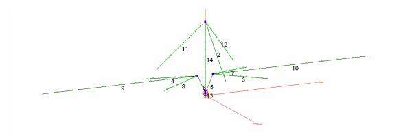
For this example the bottom of the vertical is 0.5 m off ground, 17.5m long and has three 16.6m top guys. The 160 radials are 44.9 m long and the 80 m radials are 17.8 m. An extra 5 ohm load is added in series to simulate expected ground losses. On 160 a 25 ohm inductance is added in shunt across the feed as a hairpin match. The model impedance on 160 without the hairpin is Z=9-j20 including the added 5 ohms. Adding the hairpin shunt produces this SWR curve.
