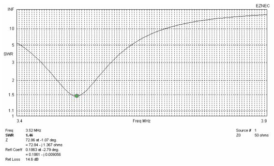
Here the model resistance at 3.525 is 73 ohms (still including the nominal 5 ohm added ground loss). At 3.8 MHz it is 132 + j366. Obviously the 366 ohms inductive can be tuned out with a smaller series C and then the SWR will have a minimum of 2.6 at 3.8 MHz.
