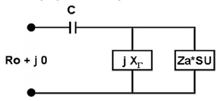
do not readily lend themselves to solutions for L, the gamma rod length and C, given Ro=Rout. However, it is easy to plot up the values of Rout and Xout =1/( $2\pi$ \*f\*C) for a range of L given d, D, f, and S. Obviously iteration methods could be used to solve for Rout(L) if desired. Here is the result of looping over a set of L values (10 to 80) to find Rout and Xout for the same d, D, f, and S used before.
