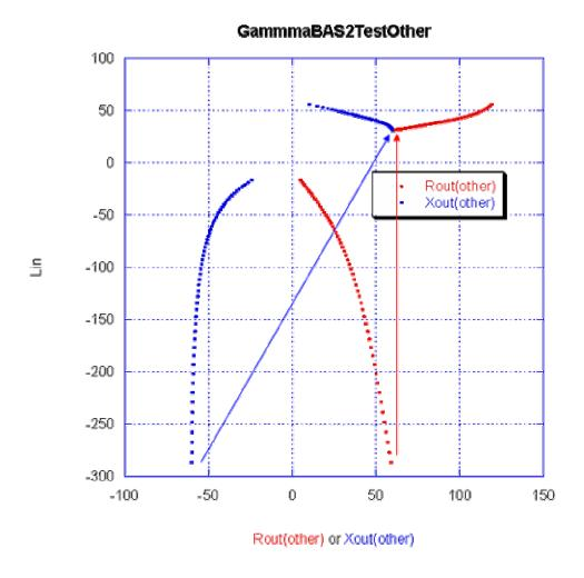
Again there is the discontinuity (arrows) at Rout=60 and the "solutions" for Rout<60, showing negative L and negative Xout, are not physical. However for Rout>60 the solutions are exactly those found when the full equations were used. To illustrate this, the last plot here is taken from "Gamma" for 0<Rout<60 and from "Gamma (other root)"
