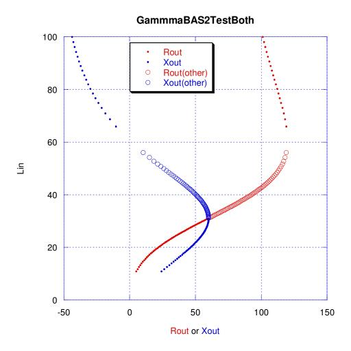
The lack of points near L=60 has no deep meaning - it was dictated by the choice of the increment of one between Rout values.
