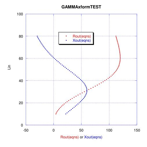
Note that there are no discontinuities, the results for Rout beyond 60 are smooth and with Xout values that are positive. Xout peaks at Rout=60. The maximum value for Rout is 120 ohms where Xout is zero. If L is made larger, Rout becomes < 120 and the Xout <0. - there may be special situations where this portion of the parameter space could be useful. But the key matter is that there exist solutions for 60<Rout<120 which are not found with the "Gamma" code.
