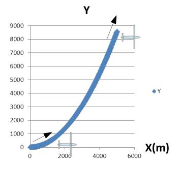
Parabolic trajectory over 100 seconds for Fv=0.
