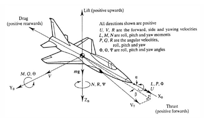
But first we will look at the equations of motion without worrying about most of the aerodynamic forces that can appear. From Fossen the parameters are given here. U,V and W are the velocity components in the **BODY** frame of reference (XB,YB,ZB) above.
